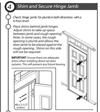
On top hinge, replace 2 short screws closest to weatherstrip with 8 x 2-1/2" screws.
